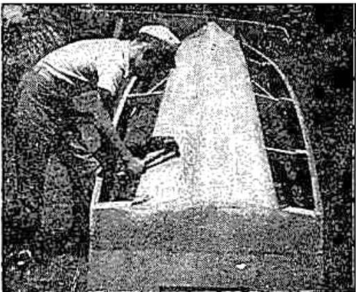
Attaching lapped bottom planks.
